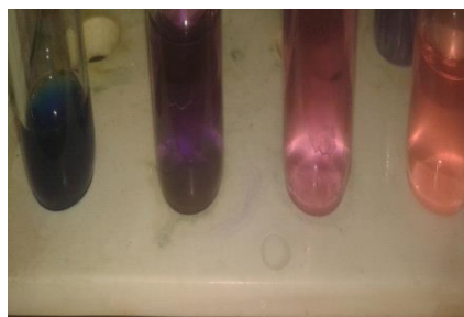
Fig. 8: Various Amines Tested with cobalt Thiocyanate
