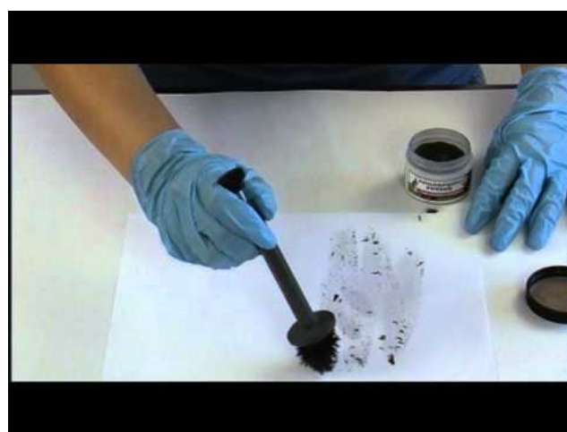
Fig. 2: Recovering fingerprints using black powder technique 6
