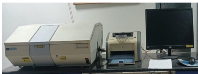
Fig. 1: Fourier transform infrared spectroscopy perkin FTIR system spectrum BX
