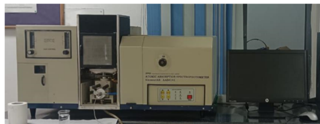
Fig. 2: Atomic Absorption Spectrophotometer Electronics of India Ltd Element AS AAS 4141
