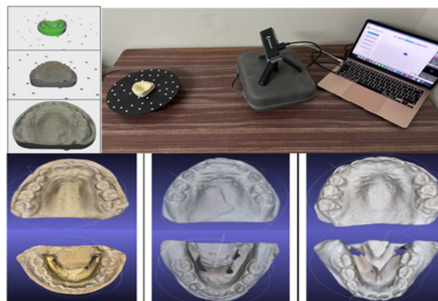
Figure 1: 3D acquisition of cast models
