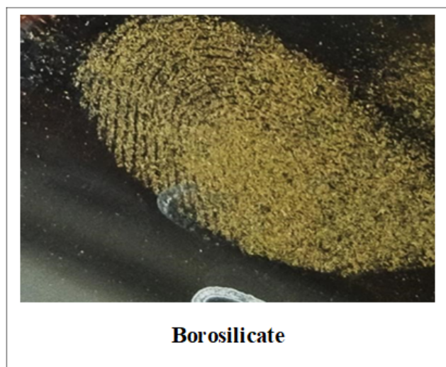
Figure 3: Visualization and development of latent fingerprints on borosilicate glass using Alternanthera leaf powder.
