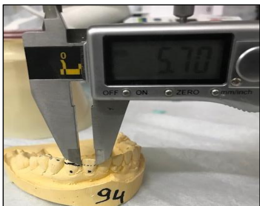
Fig. 2: Measurement on plaster
